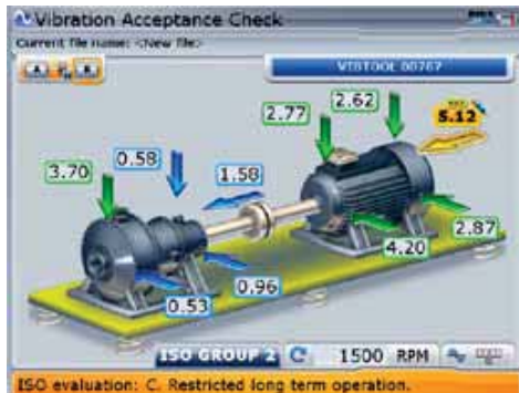
Vibration measurement results incorporated within shaft alignment program
