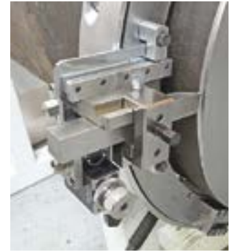
Slides feature Rapid Adjust and Micro Adjust
