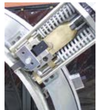
OD tracking slides follow out-of-round pipe & vessels.
