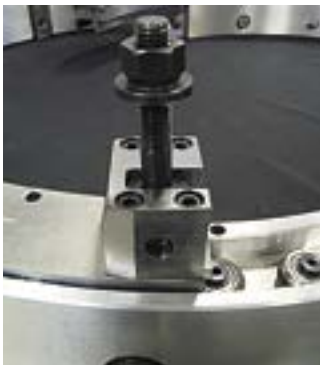
Aluminum stationary frame with steel rotating ring
