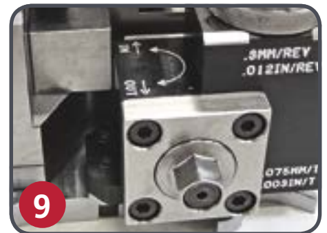
Rapid Adjust feature speeds positioning of tooling
