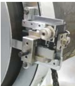
DynaPrep MDSF tool slides with Rapid Adjust
