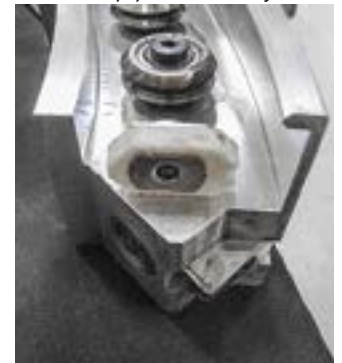
V-Lock ring mating surface resists force distortion
